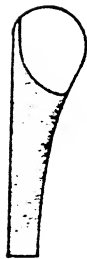
This magnified view of pen tip shows the large amount of iridium in the form of a smoothly polished ball, strongly backed up by the gold
